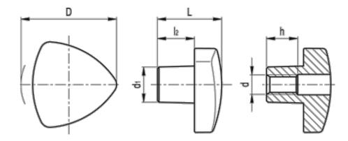
$\begin{array}{lll} D & = 32 \\ d & = M6 \\ d1 & = 12 \\ h & = 10 \\ L & = 21 \\ l2 & = 12 \\ Weight (g) = 50 \\ \end{array}$
